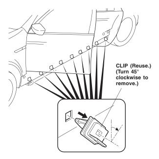
9. Assemble the left front side under spoiler and the left rear side under spoiler by inserting the ribs into the notch, and installing one clip.
