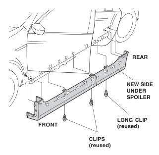
13. Reinstall the two clips and one long clip removed in step 4.
