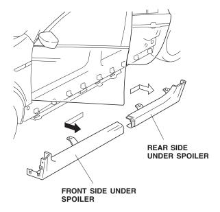
Remove the front side under spoiler by sliding it forward and out toward you. Remove the rear side under spoiler by sliding it rearward and out toward you. 7. Remove the six spring nuts from the front and rear ends of the existing side under spoilers.
