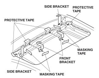
10. Set the moonroof visor on the vehicle roof and adjust its position so the holes in the visor are aligned with the side bracket holes. Install two screws and nuts loosely onto the side brackets.
