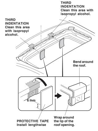
Install the protective tapes at the third indentations in from each side of the moonroof opening. Remove the adhesive backing from the protective tape and attach one at each position. Wrap 6 mm of protective tape around the lip of the moonroof opening.  Place the two front brackets and two side brackets into position over the protective tape and around the lip of the roof opening, and tape them into position with a piece of masking tape.
