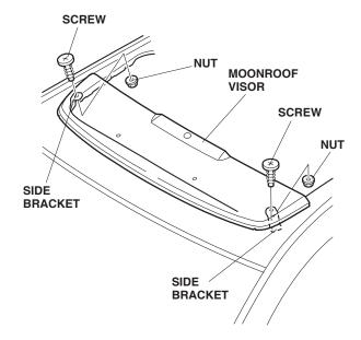
11. Align the front bracket holes with the moonroof visor holes. Install the two screws and nuts loosely onto the front brackets.
