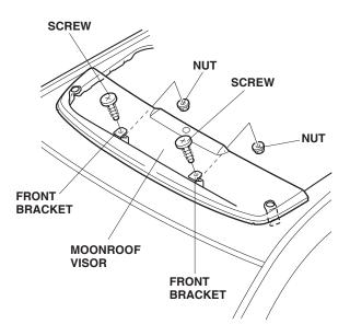
12. Position the moonroof visor with equal spacing on all sides. Check that the rubber seal is not twisted or rolled under the visor.
