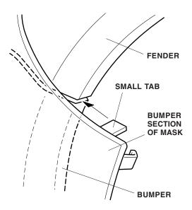
10. Attach the three plastic hooks to the inner edge of the fenderwell.
