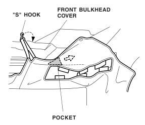
7. Attach the "S" hook to the edge of the radiator cover.
