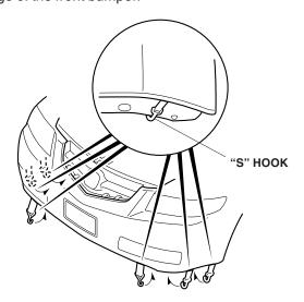
15. On each side of the vehicle, attach the snap from the mask to the snap-screws you installed in steps 4 and 5.
