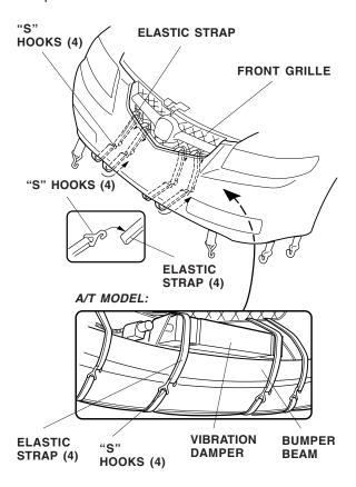
13. Attach the four "S" hooks on the bottom of the mask to the elastic straps.
