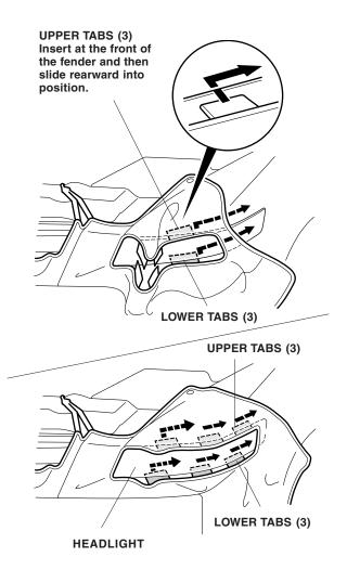
9. At the fender/bumper area, insert the small tab from the mask between the bumper and the fender.
