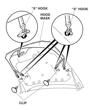
2. Fit the corners of the mask around the hood. Adjust the mask so that it fits smoothly over the edges. Attach the five "S" hooks to the hood.
