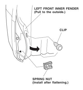
Return the left front inner fender to its original position. Get the left bracket, and install the bracket with one clip (reused) and one screw.
