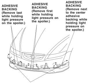
After aligning, check that there are no gaps between the spoiler and front bumper in this area.
