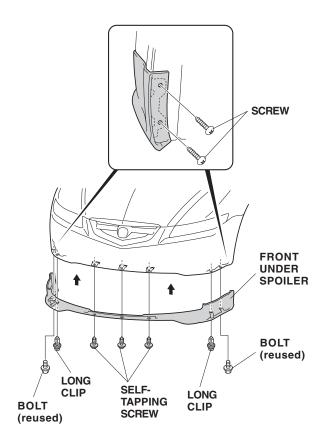
18. Position the front under spoiler on the front bumper and install it with two bolts (reused), the three self-tapping screws (supplied), four screws (supplied) and the two long clips (supplied).
