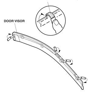
4. Attach the two front brackets of the door visor to the door sash, and push the two rear brackets over the door sash. Insert the front tab under the door mirror base.
