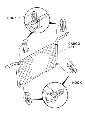
12. Install the cargo net to the tie down hooks and the anchors in the trunk. The cargo net can be installed in 2 different positions.
