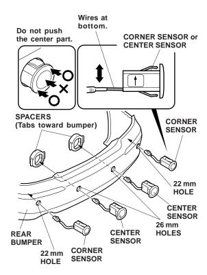
8. Slide the two center sensors into the 26 mm holes with the harness towards the bottom. Secure the two center sensors with a spacer behind the bumper. Do not push the center of the sensor; that may cause damage.
