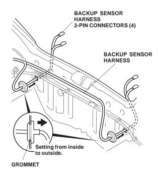
29. Seat the grommets on the backup sensor harness in the grommet holes.
