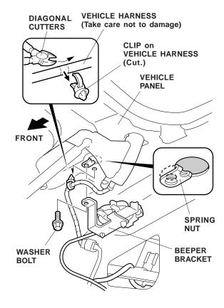
21. Install a spring nut by inserting it into the vehicle panel. Install the beeper bracket with one washer bolt. Close the trunk lid and check that the moving part of the trunk lid does not come in contact with the beeper or beeper bracket. 22. Secure the wire tie with clip to the vehicle harness. Attach the clip to the hole in the beeper bracket. Be sure to attach the wire tie with clip to the vehicle's harness in the position where you cut off the clip before.
