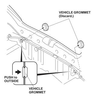
28. Continue to route the backup sensor harness (right and left) along the vehicle harness. Pull the two 2-pin connectors out through each right and left hole where the grommets were removed.
