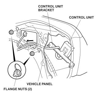
19. Plug the backup sensor harness 5-pin connector into the beeper.
