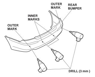
6. While wearing eye protection, drill a 22 mm hole through each of the two outer marks, and a 26 mm hole through each of the two inner marks. Remove any burrs from the edges of the holes.
