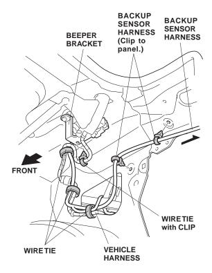
23. Route the backup sensor harness as shown. Secure the backup sensor harness to the vehicle harness with three wire ties, and attach the two clips on the backup sensor harness to the holes in the body panel as shown. 24. Remove the nut from the vehicle panel, install the short bracket, then secure it with the removed nut. Route the backup sensor harness to the rear side of the vehicle. Then attach the fuse label (2A) to the fuse case of the backup sensor harness.
