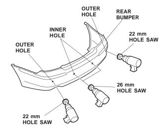
Slide the two corner sensors into the two 22 mm holes with the harness towards the bottom. Do not push the center of the sensors; that may cause damage.
