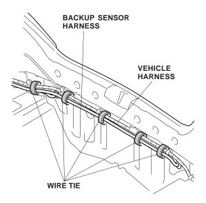
31. Cut the EPT sealer in half and attach the two halves to the backup sensor harness at each of the green tape areas. Secure the harness to the bumper beam with two wire ties.
