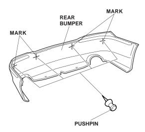
5. While wearing eye protection, drill a 3 mm hole through the four marks on the rear bumper.
