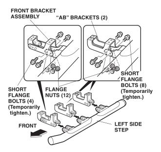
4. Adjust the location of the left side step to allow even clearance between the side step and body, then tighten the long flange bolts. Torque the long flange bolts to 27 N·m (20 lb-ft).
