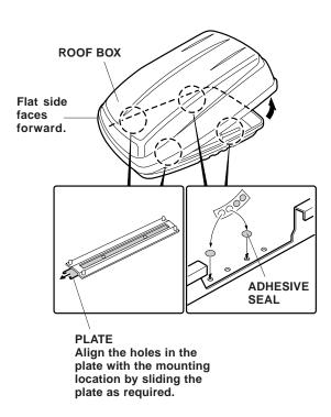
3. Attach an adhesive seal over each of the four unused mounting holes (two on each side) at the rear of the base of the box. The seals will help prevent water from entering the roof box.
