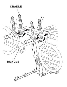
2. When loading two bicycles, alternate the direction of the bicycles.
