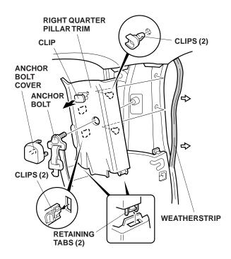
21. Remove the right rear door side sill (two clips and retaining tab). Remove the door weatherstrip around the right rear door side sill.
