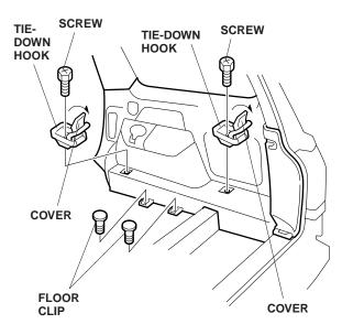
24. Remove the large plastic cover, and remove the flanged self-tapping screw under the cover. Pry out the small plastic cover with a trim tool, and remove the self-tapping screw. Pry out the small plastic cover, and remove the cargo net hook (one self-tapping screw). Remove the self-tapping screw.
