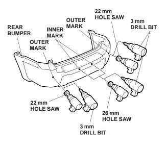
Install the two corner sensors by embedding them, as shown, in the two 22 mm holes you just made. Push only the ring at the sensor circumference. Pushing the center of the sensor could damage the sensor.
