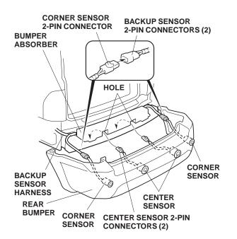
60. Connect the two outer backup sensor harness 2-pin connectors to the 2-pin connectors from the corner sensors. Reinstall the rear bumper. Check that all clips and retaining tabs are installed securely. 61. Connect the two inner backup sensor harness 2-pin connectors to the inner center sensors 2-pin connectors, then secure the 2-pin connectors to the backup sensor harness with two wire ties.
