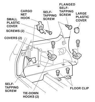
28. Remove the large plastic cover, and remove the flanged self-tapping screw concealed under the cover. Pry out the small plastic cover with a trim tool, and remove the cargo net hook (one self-tapping screw). Remove the self-tapping screw.
