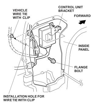
42. Install the control unit bracket in the hole for the vehicle wire tie with clip with the flange bolt.
