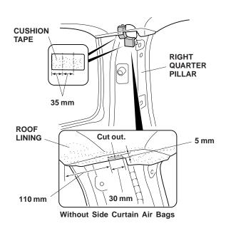
50. Using isopropyl alcohol on a shop towel, clean the area around the upper hole, then attach the cushion tape to the edge of the upper hole as shown.
