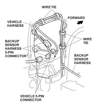
38. Unplug the vehicle 5-pin connectors, and plug them into the backup sensor harness 5-pin connectors.
