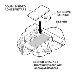
44. Using isopropyl alcohol on a shop towel, clean the inside rear panel where the beeper will attach. Remove the adhesive backing from the double-sided tape on the beeper, and attach the beeper to the inside rear panel. You must have 5 mm of clearance between the 5-pin connector and the edge of the inside rear panel. Hold the beeper in place for 30 seconds.
