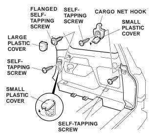
25. Remove the tailgate weatherstrip in the area shown. Remove the eight clips and the four retaining tabs, unplug the vehicle connector from the AV jack terminal (if equipped), and remove the right rear side panel.
