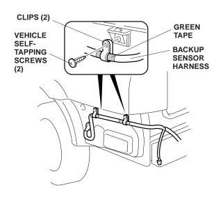
34. Attach the four wire ties with clip to the backup sensor harness where the green tape is located, then push the clips into the holes in the bumper beam and body frame. If a trailer hitch is installed, cut the clip off the wire tie with clip, align the green tapes on the trailer hitch and backup sensor harnesses, and then secure the harnesses with the wire tie.
