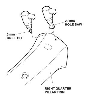
57. Pull the backup sensor harness 4-pin connector out through the 20 mm hole, then reinstall the right quarter pillar trim. Check that all clips and retaining tabs are installed securely.
