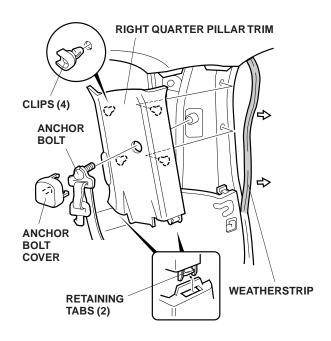
20. Remove the right quarter pillar trim (four clips and two retaining tabs).
