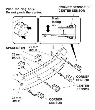
14. Install the two center sensors into the 26 mm holes. Install the two center sensors by embedding them, as shown, in the two 26 mm holes you just made. Secure the center sensors with one spacer for each sensor. Push only the ring on the sensor circumference. Pushing the center of the sensor could damage the sensor.
