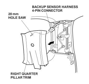
58. Plug the backup sensor harness 4-pin connector into the switch, then install the switch into the hole in the right quarter pillar trim, in the direction shown.
