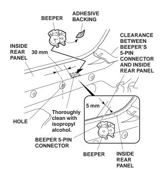
45. Plug the backup sensor harness 5-pin connector into the beeper 5-pin connector.
