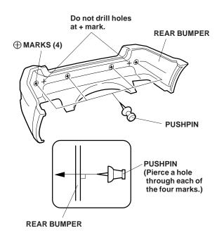
12. While wearing eye protection, drill a 22 mm hole through each of the two outer marks, and a 26 mm hole through each of the inner marks. Remove any burrs from the edges of the holes. First drill with a 3 mm drill bit, and then finish with a 22 mm hole saw or a 26 mm hole saw.
