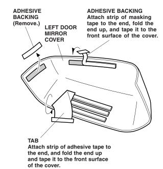
Attach strips of masking tape to the ends of the upper adhesive backing and center tab. Fold those ends up, and temporarily tape them to the surface of the door mirror cover. Remove the remaining adhesive backings.
