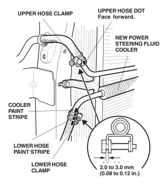
10. Align the paint stripe on the lower hose with the paint stripe on the cooler, then tighten the lower hose clamp to the specification shown.
