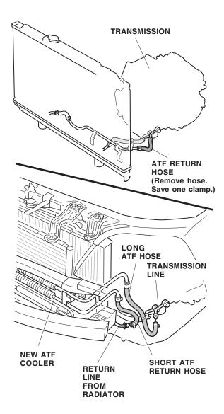
14. Attach the long ATF hose to the transmission line where you removed the return hose using one new hose clamp.
