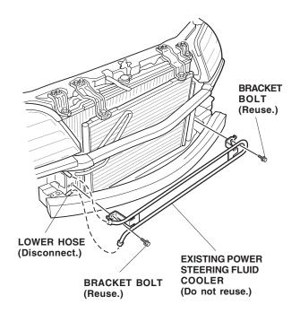
8. Attach the lower hose to the new power steering fluid cooler, and fit the cooler into position on the front bulkhead. Reinstall the two bracket bolts, and torque the bolts to 11 N·m (8 lb-ft).
