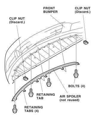
2. Remove the two bolts and five clips from the bottom of the front bumper.
