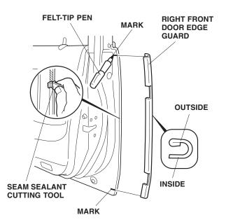
5. Position the cutting edge of the seam sealant cutting tool against the door edge, and trim the seam sealant between the marks at the top and bottom of the door edge.
