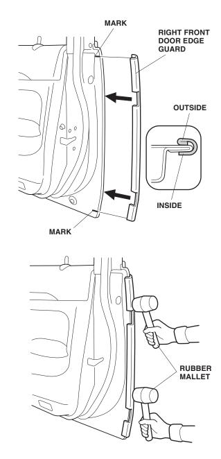
8. Repeat steps 3 thru 7 to install the left front door edge guard.
