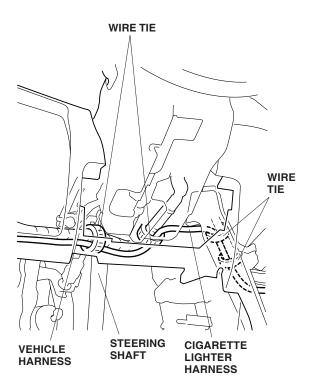
14. Continue routing the cigarette lighter harness to the center console opening, and secure it to the vehicle harness with the five wire ties.
