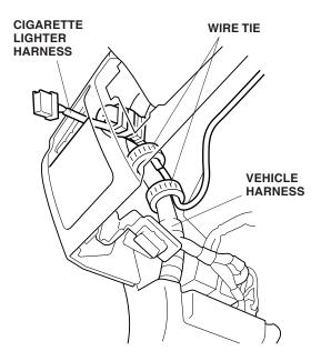
12. Plug the cigarette lighter 5-pin connector into the VSA switch, and reinstall the switch panel.
