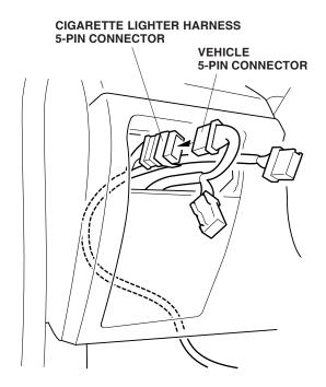
11. Route the other end of the cigarette lighter harness along the vehicle harness, and secure it to the vehicle harness with two wire ties in the areas shown.
