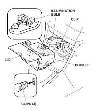
5. Remove the four self-tapping screws. Gently pull out on the coin pocket holder, unplug the vehicle connector and vehicle clip, and remove the coin pocket holder.
