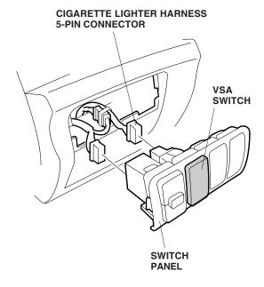
13. Route the cigarette lighter harness in front of the steering shaft. Secure the cigarette lighter harness to the vehicle harness with four wire ties.
