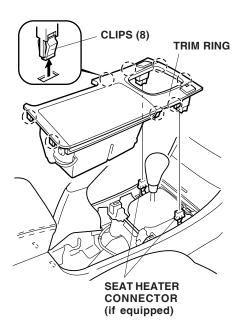
4. Open the pocket lid. Pull the pocket out toward you to release the four clips, unplug the illumination bulb, unclip the illumination bulb harness from the pocket, and remove the pocket. Tack care not to damage the illumination bulb.
