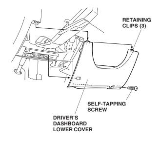
7. Remove the driver's dashboard under cover (three clips, one pin and one holder).
