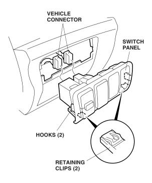
9. Unplug the vehicle connectors from the switch panel, then remove the switch panel.
