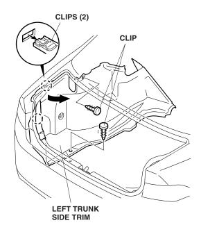
Pull the left trunk side trim out in the direction shown. While wearing eye protecetion, drill a 15 mm hole through the left trunk side trim at the mark using a hole saw. Take care not to damage the inner panel and wire harnesses under the trim.
