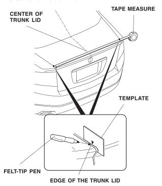
4. Measure 278 mm (10.9 in.) outboard from the center and mark the trunk lid on each side. Position the template on the trunk lid. Using a felt-tip pen, mark the trunk lid as indicated on the template. Do this procedure on each side of the trunk lid.
