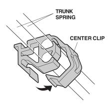
16. With an assistant holding the trunk lid open, remove the old left trunk springs from the trunk hinge arms using the special tool. Wear gloves to protect your hands, and pull the special tool slowly and carefully toward you.
