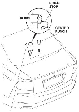
DRILL First drill with a 3 mm drill bit, and finish with an 8 mm drill bit.
