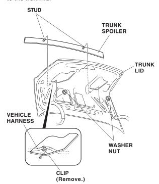
9. Fit the spoiler into position on the trunk lid by inserting the two studs into the holes in the trunk lid. With an assistant holding the trunk lid open, install a flange nut on the end of each stud. Install the two washer-bolts, but do not tighten them yet. 10. When the trunk spoiler is aligned properly with the trunk lid, carefully remove the adhesive backing on each side. Hold the spoiler firmly against the trunk lid with the palm of your hand.
