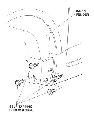
3. Position the left front splash guard on the left inner fender, with the tang from the splash guard around the side sill. Reinstall the four self-tapping screws.
