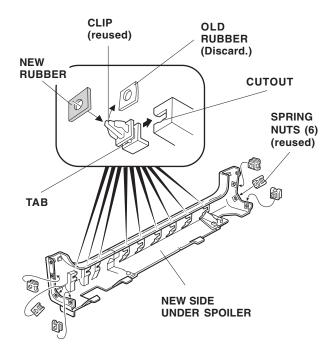
11. Install the six spring nuts removed in step 7 onto the front and rear ends of the new side under
