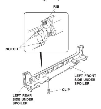
10. Slide the nine clips (removed in step 8) into the holders on the new side under spoiler through the slots, and align the tabs on the clips with the cutouts on the holders shown. Remove the existing rubber spacers from the clips and install a new rubber spacer onto each of the nine clips.
