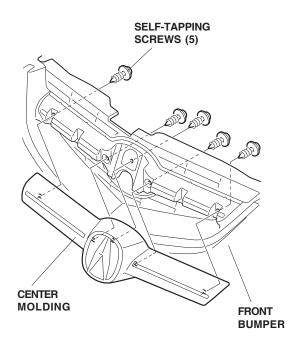
8. Remove the two self-tapping screws that secure the existing "A" emblem and remove the emblem.
