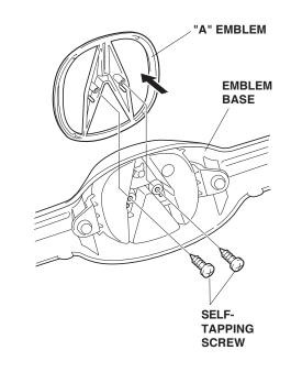
9. Slide the pins on the gold "A" emblem into the holes in the emblem base and install the two self-tapping screws you just removed.
