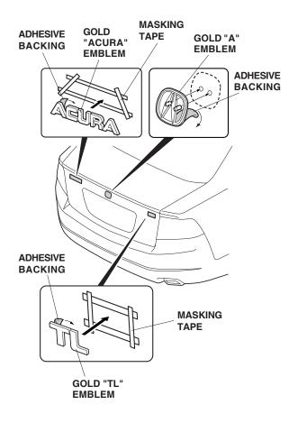
16. Remove the masking tape installed around the emblems in step 10.
