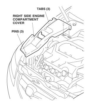
5. Open the engine hood. Remove the front bulkhead cover (three clips, two screw clips and two pins).
