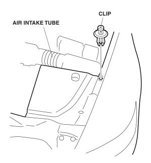
4. Install one new clip with a snap-screw into the hole where you removed the clip, and tighten the snap-screw.
