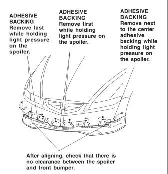
21. Hold the spoiler firmly against the front bumper with the palm of your hand for 30 seconds, particularly at the edges.
