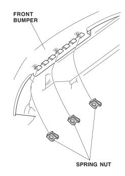
6. Position the left cover on the front bumper and align the end of the cover with the edge of the bumper. Mark the center of each circle through the left cover with a felt-tip pen.
