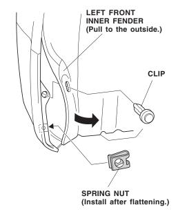
14. Return the left front inner fender to its original position. Get the left bracket, and install the bracket with one clip (reused) and one screw.
