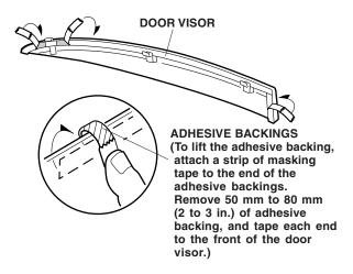
11. Attach the rear bracket of the door visor to the door sash, and push the two front brackets on the door sash.
