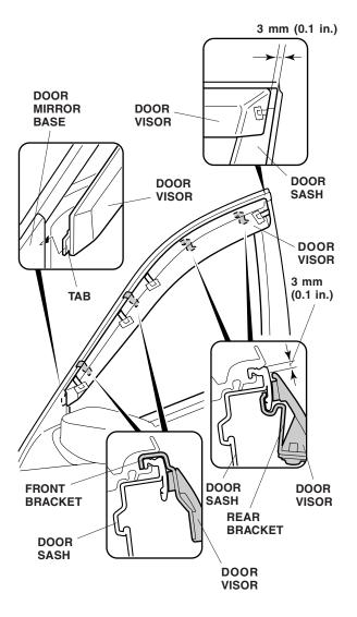
5. Adjust the location of the door visor so that the clearance between the door visor and door sash is 3 mm (0.1 in.) at the top, and 3 mm (0.1 in.) at the back. There should be no clearance between the front tab and the visor.
