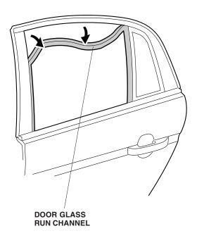
9. Using isopropyl alcohol on a shop towel, clean the shaded area of the door sash.
