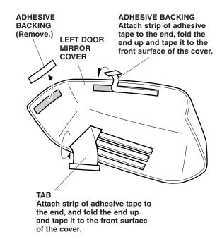
Attach strips of masking tape to the ends of the upper adhesive backing and center tab. Fold those ends up and temporarily tape them to the surface of the door mirror cover. Remove the remaining adhesive backings.
