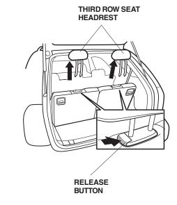
Store the headrests in the storage compartment under the cargo floor. Insert the shafts of the headrests into the holes in the sides of the storage compartment.
