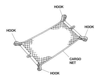
6. Attach the hooks to the anchors in the cargo area.
