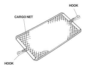
8. Fold the cargo net in half, attach the hooks to the anchors in the floor, and attach the loops to the hooks on the side panel.
