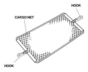
8. Attach the hooks to the anchors in the floor, and attach the loops to the hooks on the side panel.
