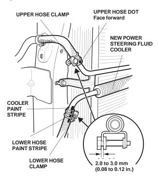
Align the paint stripe on the lower hose with the paint stripe on the cooler, then tighten the lower hose clamp to the specification shown.
