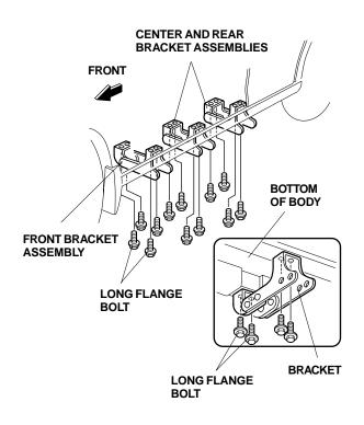
Install the left side step to the bracket assemblies using 12 short flange bolts and 12 flange nuts. Torque the flange bolts to 24 N•m (18 lb-ft).
