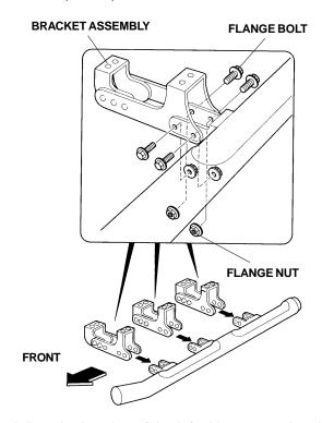
Adjust the location of the left side step so that the clearance is even between the side step and the body. Torque the short flange bolts you installed in steps 1 and 2 to 24 N•m (18 lb-ft).
