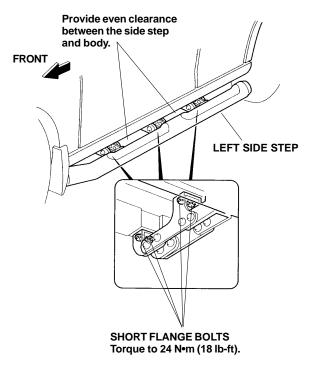
6. Repeat steps 1 through 5 to install the right side step on the vehicle.
