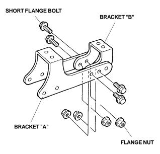
At the left side of the vehicle, install one bracket assembly at the front, one at the center, and one at the rear along the body using 12 long flange bolts. Thread the long flange bolts in about 3 or 4 threads.
