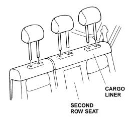
6. Install the cargo liner over the second row seats, then reinstall the headrests.
