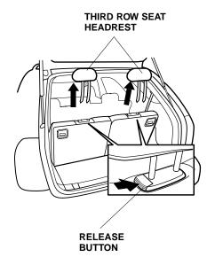
Store the headrests in the storage compartment under the cargo floor. Insert the shafts of the headrests into the holes in the sides of the storage compartment.
