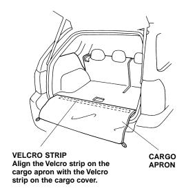
23. Attach the loops of the cargo apron to the vehicle hooks in the cargo area.
