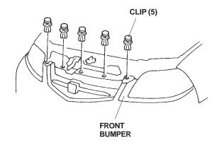
Remove the two self-tapping screws, the two clips, and the four bolts that secure the front bumper.
