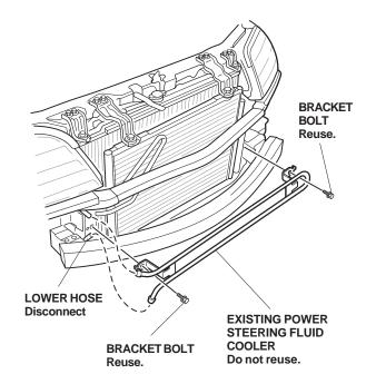
Attach the lower hose to the new power steering fluid cooler, and fit the cooler into position on the front bulkhead. Reinstall the two bracket bolts, and tighten them securely.
