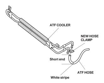
12. Route the hose installed on the ATF cooler through the bulkhead, and fit the ATF cooler into position on the front bulkhead. Install the two 6 x 12 mm washer-bolts from the kit through the ATF cooler and into the threaded holes in the front bulkhead. Tighten the bolts securely.
