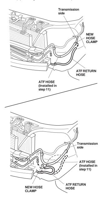
14. Attach the ATF hose (installed in step 11) to the transmission side where you removed the return hose using one new hose clamp.
