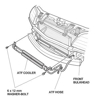
13. Remove the ATF return hose from the transmission side, and attach the return hose to the lower ATF cooler pipe using one new hose clamp.
