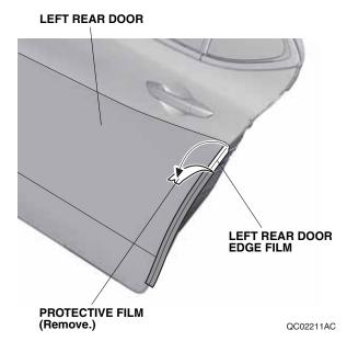
21. Starting from the center and working outward, use your fingers to fold the door edge film inside the door. Move your fingers in one direction only. Do not damage the door seam sealant.
