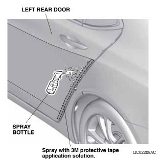
17. Open the left rear door. Peel back about 50 mm (2.0 in.) of adhesive backing from the left rear door edge film. Align the top edge of the protective film with the bottom of the character line, and the V-notch with the door edge.
