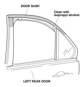
20. Position the left rear door visor on the door sash.
