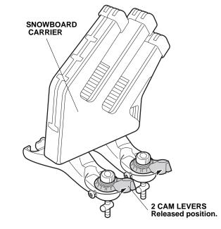
5. Attach the two bottom clamps to the top clamps.
