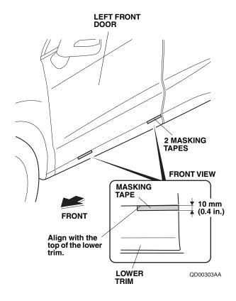
Using one alcohol swab, thoroughly clean the left front door where the left front lower chrome trim will attach.
