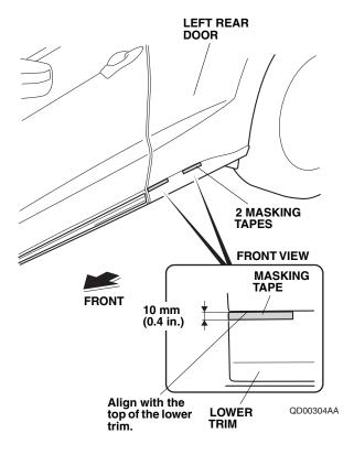
8. Using one alcohol swab, thoroughly clean the left rear door where the left rear lower chrome trim will attach.
