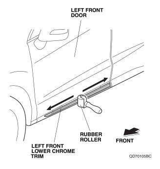
7. Attach the masking tapes to the lower trim as shown.
