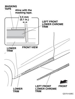
5. While applying light pressure against the left front lower chrome trim, carefully remove the adhesive backings.
