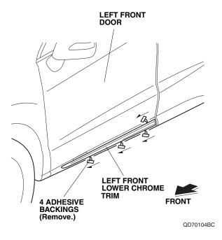
6. Using a rubber roller, apply firm pressure against the left front lower chrome trim and roll from one end to the other. Apply firm pressure especially at the ends.
