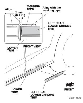
While applying light pressure against the left rear lower chrome trim, carefully remove the adhesive backings.
