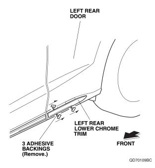
12. Using a rubber roller, apply firm pressure against the left rear lower chrome trim and roll from one end to the other. Apply firm pressure especially at the ends.
