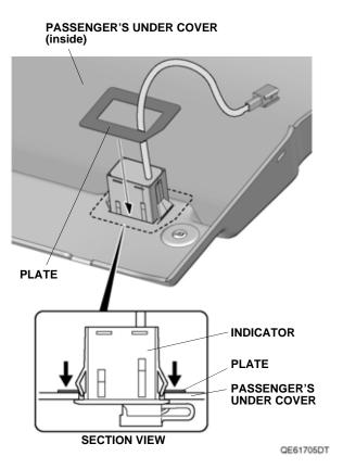
10. Secure the green tape section of the indicator harness to the passenger's under cover with one wire tie.
