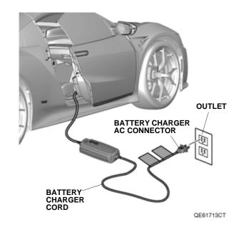
24. Monitor the battery charger status indicator lights. If the RED error light is on, refer to the Battery Charger User's Information Manual for troubleshooting. If the charging lights are progressing continue on to step 25.
