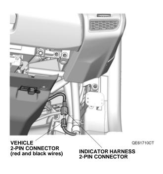
15. Secure the 2-pin connectors and the indicator harness to the vehicle harness with two wire ties.
