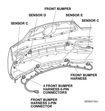
33. Secure the two front bumper harness clips to sensor D and sensor E as shown.
