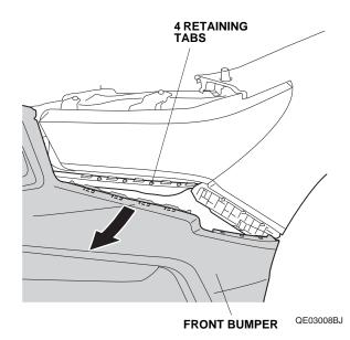
• With the help of an assistant, release the front bumper. Place the front bumper on the blanket to prevent damage.
