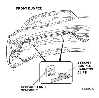
34. Secure the six front bumper harness clips to the front bumper as shown.
