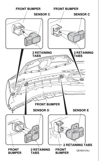
32. Plug the four front bumper harness 6-pin connectors into sensor D, sensor E and both sensors C.
