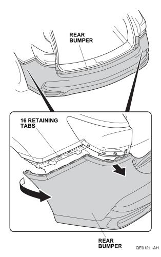
With the help of an assistant, remove the rear bumper. Place the rear bumper on a blanket to prevent damage.
