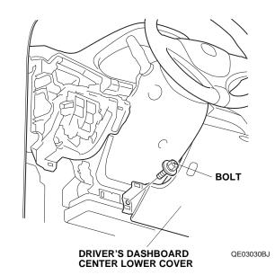
13. Remove the driver's dashboard center lower cover and unplug the vehicle connector and temperature sensor.
