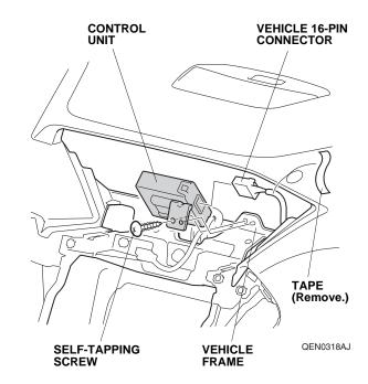
38. Attach the control unit to the vehicle frame using the self-tapping screw.
