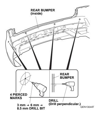
22. Using the 16 mm Punch Tool, punch out the four rear bumper holes as shown.
