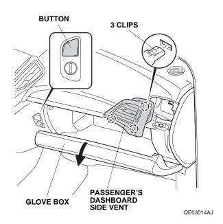
4. Remove the passenger's dashboard trim panel. Close the glove box.
