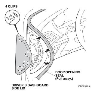
8. Remove the driver's dashboard side vent.
