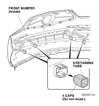
31. Attach two sensors C, one sensor D, and one sensor E to the front bumper as shown.
