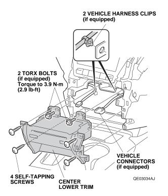
15. Loosen the two bolts as shown. Remove the audio unit assembly and unplug the vehicle connectors.
