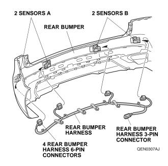
27. Secure the four rear bumper harness clips to the two sensors A and two sensors B as shown.
