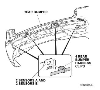
28. Secure the four rear bumper harness clips to the rear bumper as shown.
