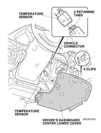
14. Remove the center lower trim and unplug the vehicle connectors.
