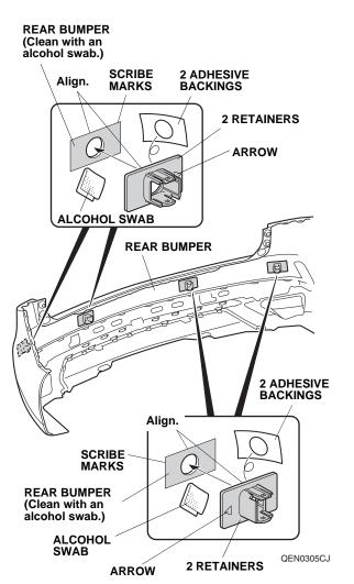
24. Attach the four retainers to the rear bumper as shown.
