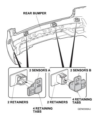
26. Plug the four rear bumper harness 6-pin connectors into the two sensors A and the two sensors B.
