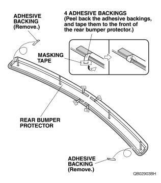
11. Align the rear bumper protector to the rear bumper as shown, and attach it to the rear bumper as shown.
