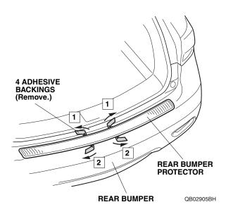
13. Using a rubber roller, apply firm pressure to the rear bumper protector, especially at the ends, as shown.
