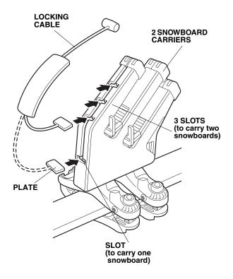
14. After loading the snowboards on the carrier, adjust them with the help of the board supports so that the top edges are level and the boards are as far down in the carrier as possible. To secure the snowboards, use the key to open the covers, then insert the locking cable barrels into the holes in the carrier covers.
