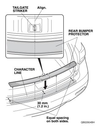
12. While applying light pressure against the rear bumper protector, carefully remove the adhesive backings in the order as shown.
