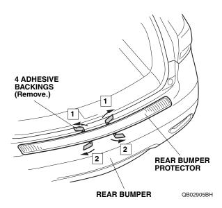
Using a rubber roller, apply firm pressure to the rear bumper protector, especially at the ends, as shown.
