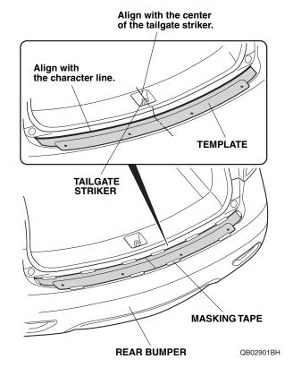
6. Using a pushpin, pierce four marks through the template as shown.
