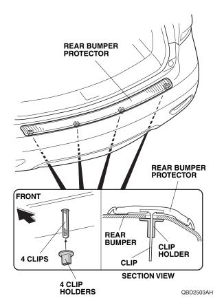
15. Reinstall the all removed parts.
