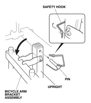
2. Reinstall the pin and safety hook as shown.
