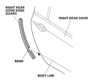
Using a felt-tip pen, mark the inside edge of the right rear door at the upper and lower ends of the right rear door edge guard.
