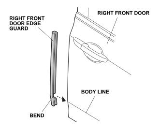
2. Using a felt-tip pen, mark the inside edge of the right front door at the upper and lower ends of the right front door edge guard.
