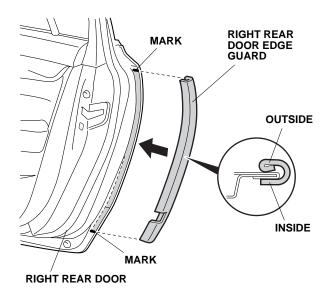
14. Using a rubber mallet, lightly tap on the right rear door edge guard.
