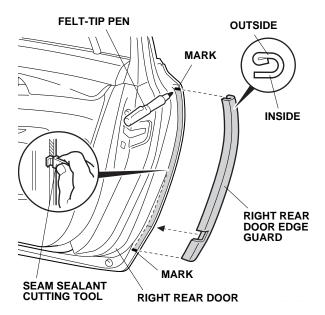
11. Position the cutting edge of the seam sealant cutting tool against the door edge, and trim the seam sealant between the marks at the top and bottom of the door edge.
