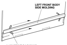
2 ADHESIVE BACKINGS Press on the left front body side molding firmly with the palm of your hand while removing the adhesive backings.
