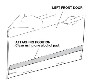
4. Align the edges of the left front body side molding with the edges of the front template as shown, then install the left front body side molding on the left front door.
