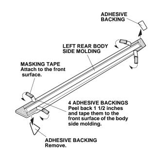
10. Using one alcohol pad, clean the door surface where the left rear body side molding will attach. Allow the alcohol to dry.
