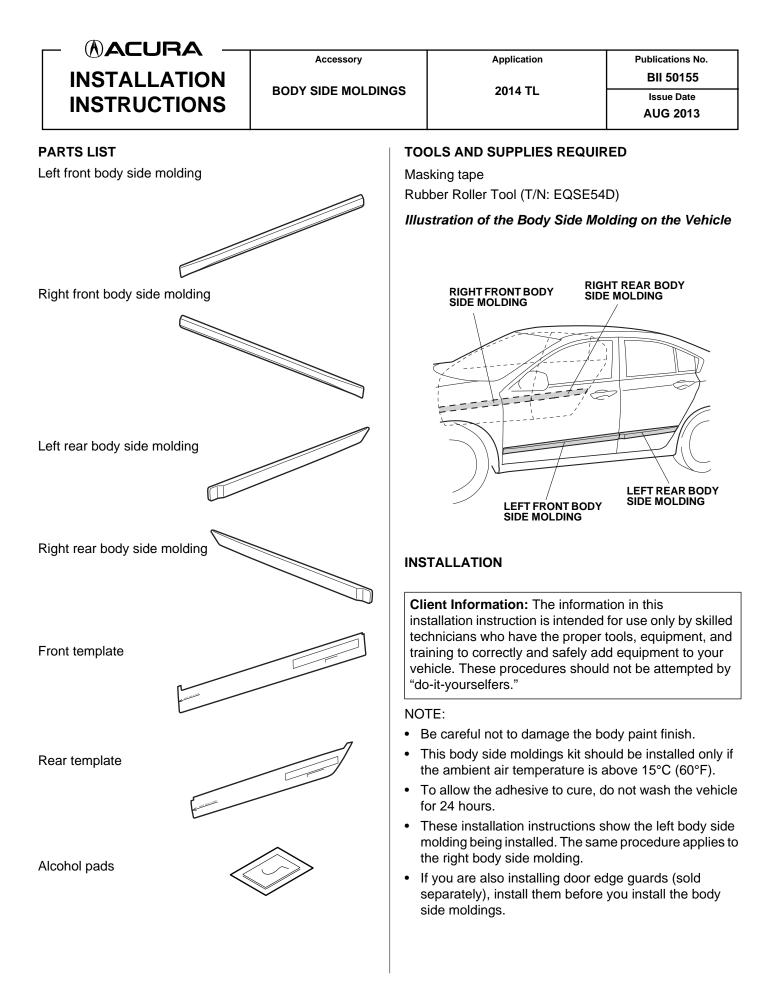
1. Position the front template on the door, and align its edges with the edges of the left front door. Secure the template with masking tape as shown.
