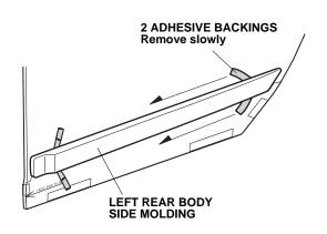
13. Using the rubber roller, apply firm pressure while rolling to set the adhesive.
