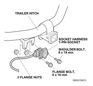
11. With the help of an assistant, position the trailer hitch on the vehicle and loosely install the six flange bolts.
