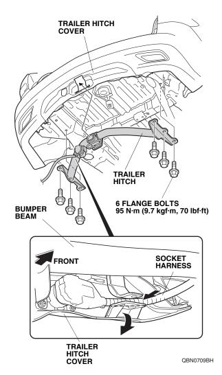
12. Torque the six flange bolts to 95 N·m (9.7 kgf·m, 70 lbf·ft).
