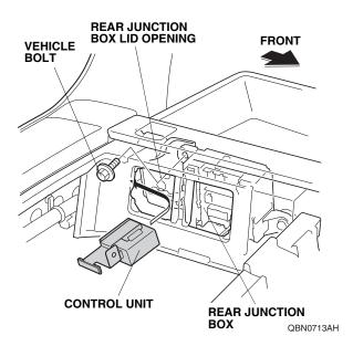
20. Position the control unit bracket as shown, and secure the control unit bracket with the vehicle bolt.
