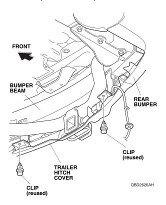
14. Using isopropyl alcohol on a shop towel, thoroughly clean the trailer hitch cover where the caution label will attach.
