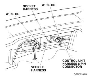
36. Secure the socket harness to the vehicle harness with one wire tie.
