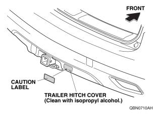
15. Attach the caution label to the trailer hitch cover at the area shown.
