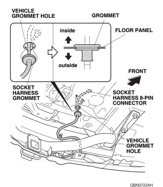
31. Secure the socket harness clip to the vehicle frame.
