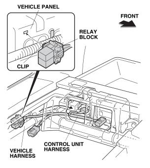
23. Plug the control unit harness 14-pin connector into the rear junction box 14-pin connector.
