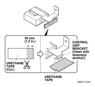
18. Using scissors, cut one urethane tape to the measurement shown. Wrap the cut urethane tape to the control unit bracket as shown.
