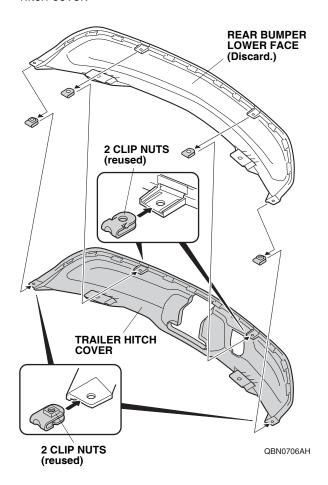
Install the trailer hitch cover to the rear bumper.
