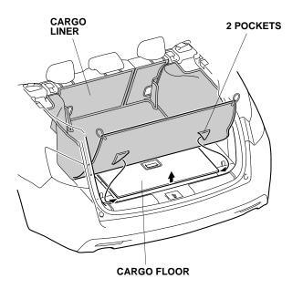
5. Insert two tabs on the cargo liner between the left side trim.
