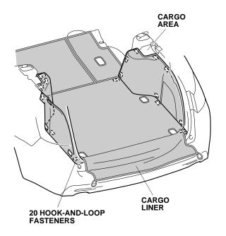
10. Secure two loops on the cargo liner to two hooks.
