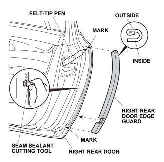
11. Position the cutting edge of the seam sealant cutting tool against the door edge, and trim the seam sealant between the marks at the top and bottom of the door edge.
