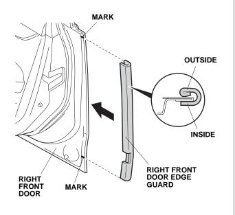
6. Using a rubber mallet, lightly tap on the right front door edge guard.
