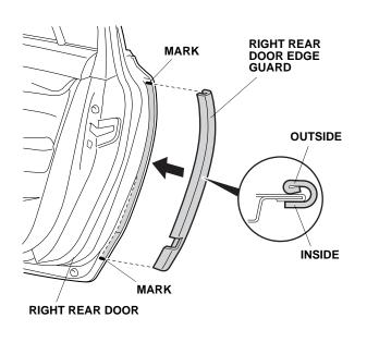
14. Using a rubber mallet, lightly tap on the right rear door edge guard.
