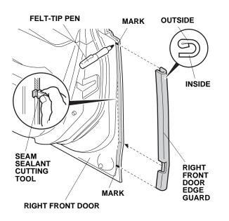
3. Position the cutting edge of the seam sealant cutting tool against the door edge, and trim the seam sealant from mark to mark.
