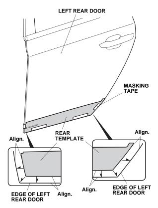
Peel back approximately 1½ inches of the adhesive backing from each adhesive strip, and tape the ends to the front surface of the left rear body side molding. Remove the small end pieces of adhesive backing.
