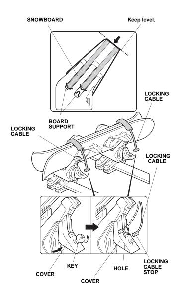
16. Check that the locking cables are installed securely, then close the covers.
