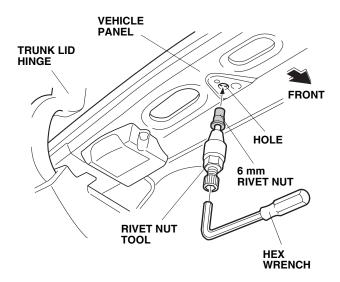
3. Hold the rivet nut tool with the hex wrench, and turn the 19 mm wrench clockwise to install the 6 mm rivet nut into the vehicle panel.
